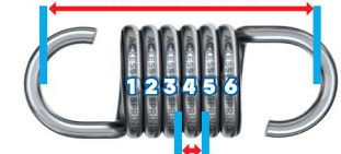
WIRE DIAMETER THIS SPRING HAS 6 TOTAL COILS
